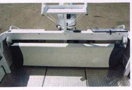
Power: The Morningstar 460 Cuddy Sports Angler is rated for single, long-shaft outboard 40-90hp. However, after testing the boat with a single Honda 60hp I wouldn't think you would want to go for anything smaller than the 60-size motor.
