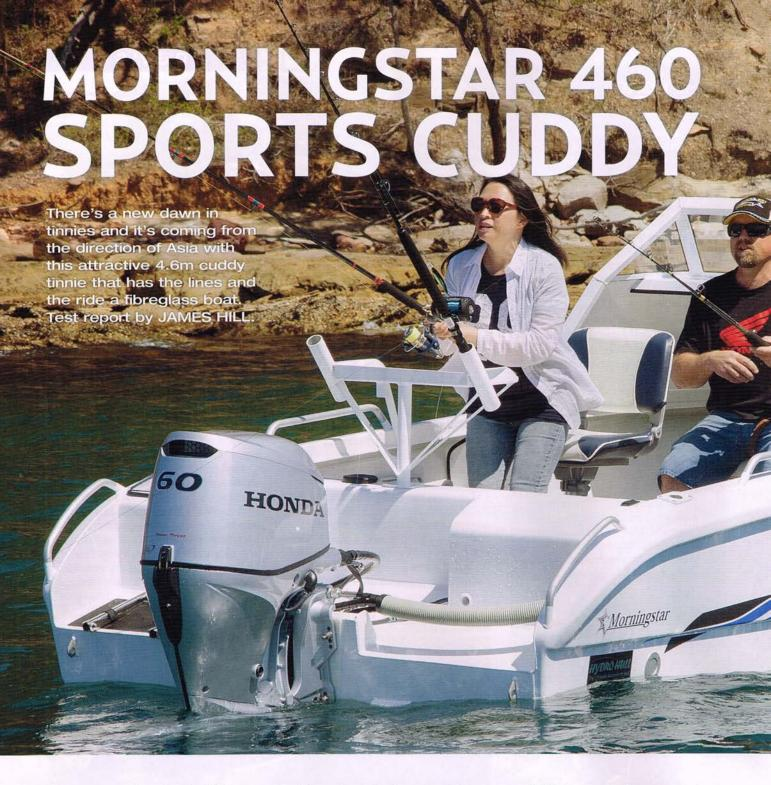
ast year we introduced *TBF* readers to a small console craft from Asia that really does offer something different for tinnie boat buyers. Indeed, the Morningstar 460 is more akin to a fibreglass boat due to its innovative construction that has each side of the boat and deck pressed from one sheet under massive load.
